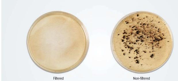
Filtered samples won't clog your pipette, and allow for clean plating so that you can count colonies instead of debris.
